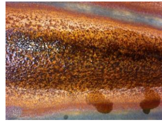
^ Owatrol applied directly to tight rust
